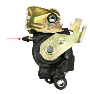
When bleeding this type of parking brake caliper where the bleeder screw is horizontal once installed, we have found that they bleed best when the bleeder screws are **parallel to the ground**. If it is not, then it will be necessary to reposition the vehicle, the axle, or the caliper. **If the bleeder screw is not parallel to the ground while bleeding, then you can bleed gallons of fluid through it without eliminating all of the air.**
