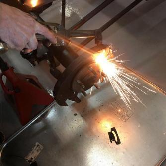
Disconnect and remove the parking brake cable and lever. The brackets in this kit are designed to be installed without removing the differential cover. This can be done by use of a cut-off wheel, reciprocating saw, or torch to split the backing plate into two pieces for removal. If you wish to retain your backing plates, the axles can be removed from the housing by draining the fluid, then removing the differential cover and the axle shafts.
