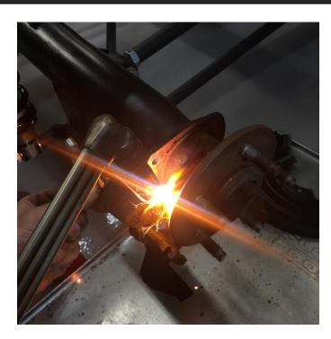
Remove the original caliper mounting bracket. Again, this can be done using any method you prefer.
