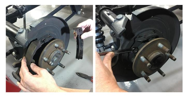
Once the disc is removed, remove all springs retaining the stock shoes and discard them. Next, unbolt the backing plate from the axle flange.
