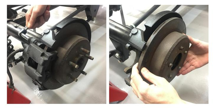
This installation refers to the **passenger side** of the axle (unless noted). All steps are to be repeated on the driver side. Start by removing the factory caliper and disc. It may be necessary use a lubricant around the axle register to do this, if corrosion is present.
