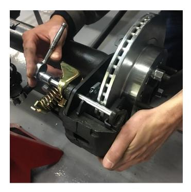
The calipers can now be installed using medium strength threadlocker (such as Loctite 243) on the threads of the two 7/16-20 caliper bolts and torque to **30 ft-lbs**. For parking brake calipers, refer to the instructions below for Parking Brake Caliper Setup
